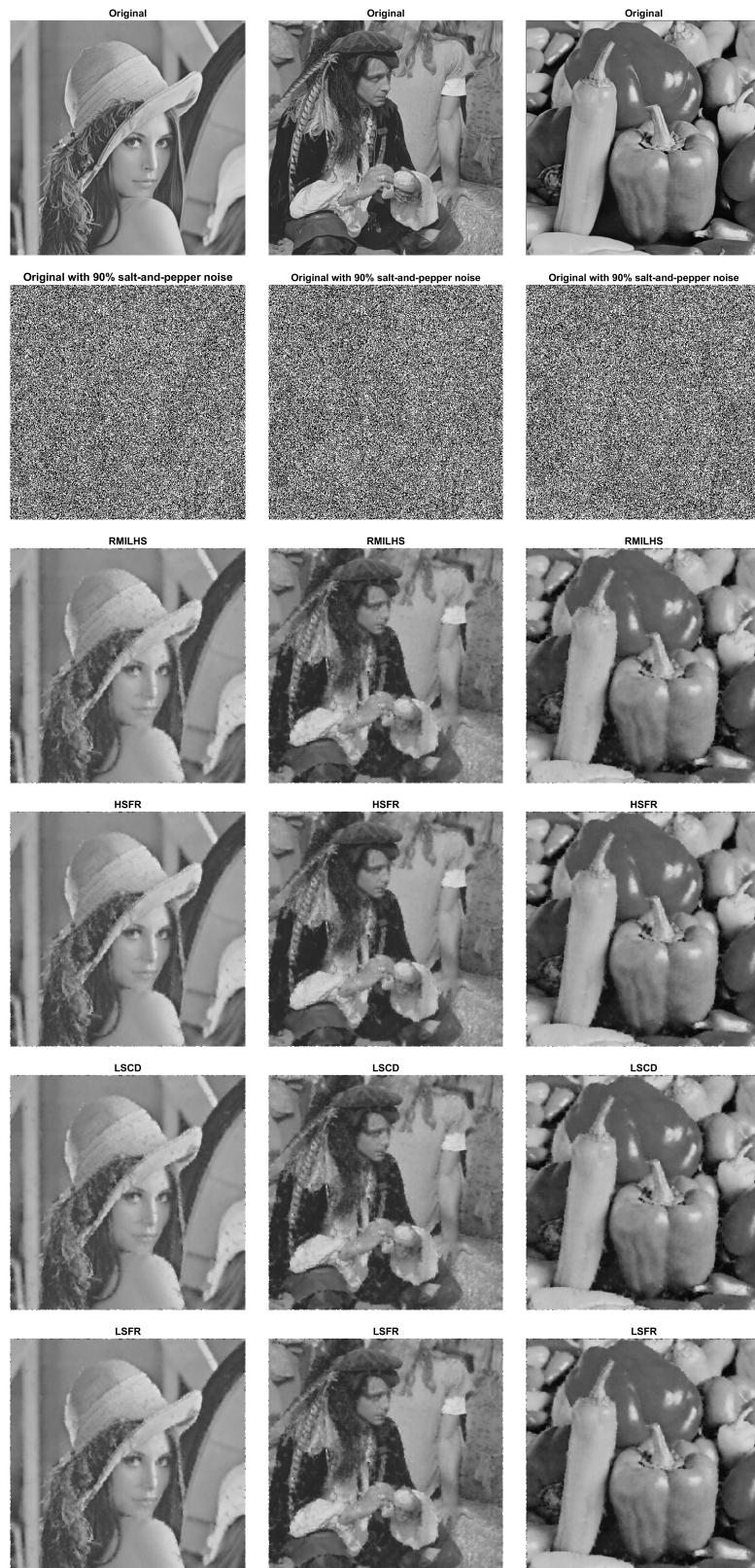
Figure 2.5: The original images, the noisy images with 90% salt-and-pepper noise and the restored images by RMILHS , HSFR, LSCD and LSFR.
