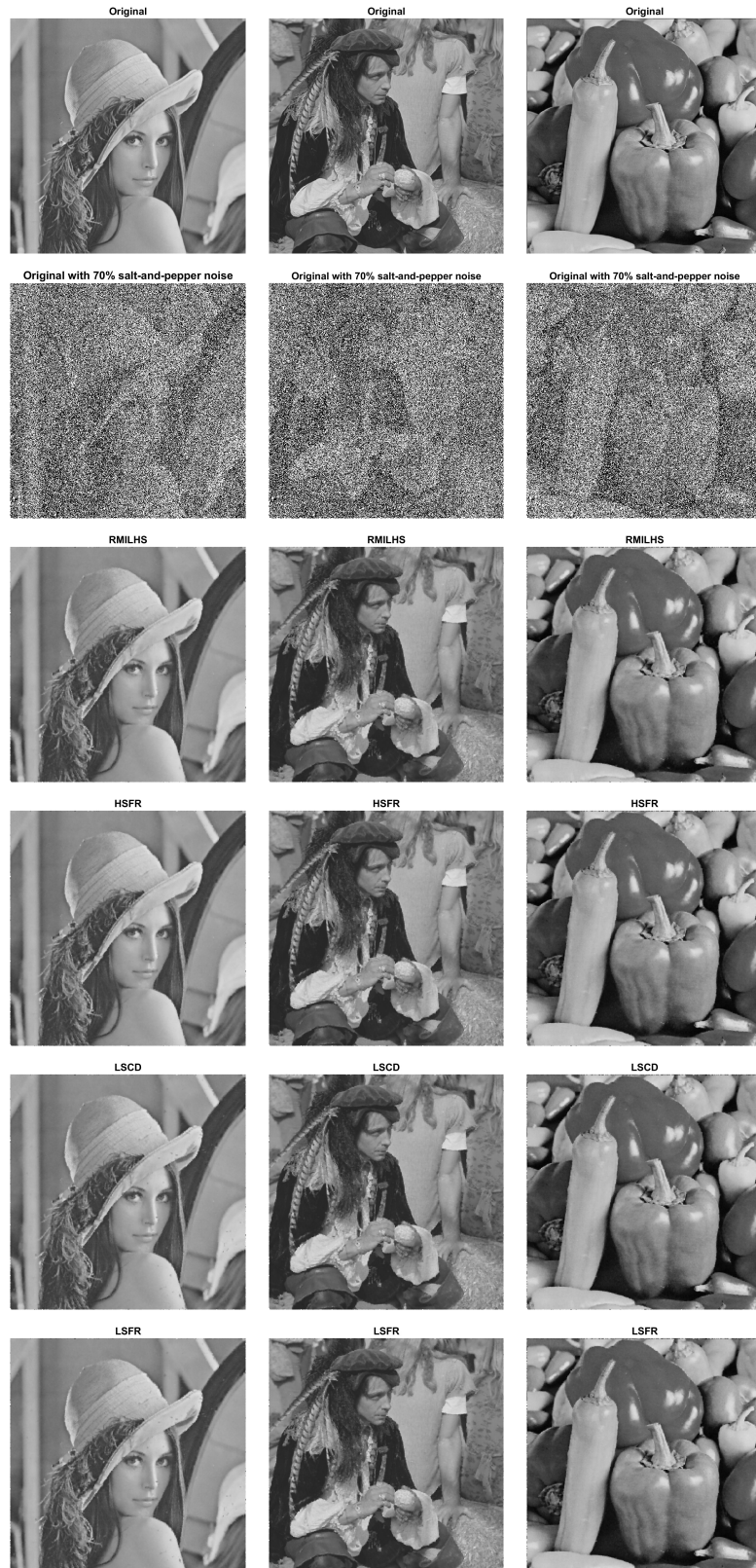
Figure 2.4: The original images, the noisy images with 70% salt-and-pepper noise and the restored images by RMILHS , HSFR, LSCD and LSFR.
