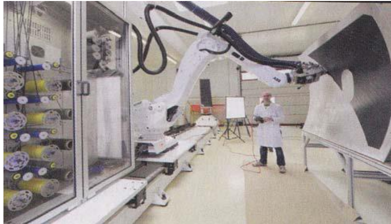
Figure I. 10: Robot system lays thermoset, thermoplastic or dry fiber[31]
