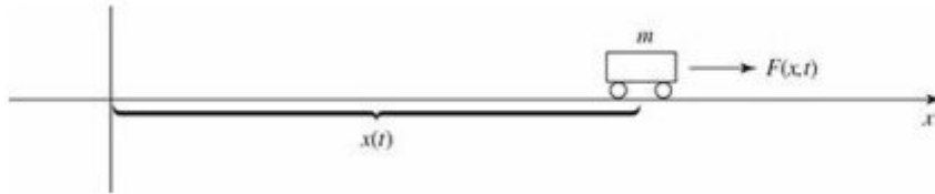
Figure :1.8 A “particle” constrained to move in one dimension under the influence of a specified force.
