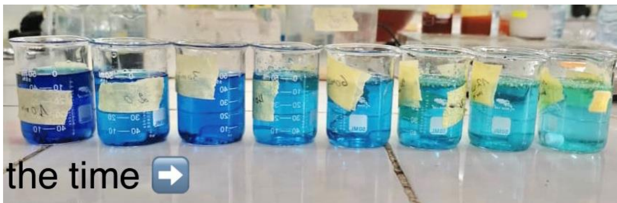
Figure 8. Sequence of digital photographs proving MB adsorption with Cs material.
