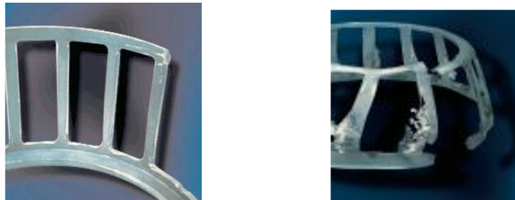
Figure 1.17 - Rupture de la cage
